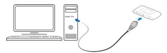
3. After charging, remove the USB cable from both the hotspot and the computer.
