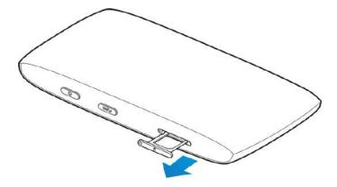
3. Hold the replacement nano-SIM card with the contacts facing upwards and place it into the tray.
