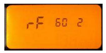
That's the setting to indicate the speedlights are set for the YN603 series transceivers. Note the strange spacing between "60" and the number "2" in the LCD and you'll know why I was so confused.
