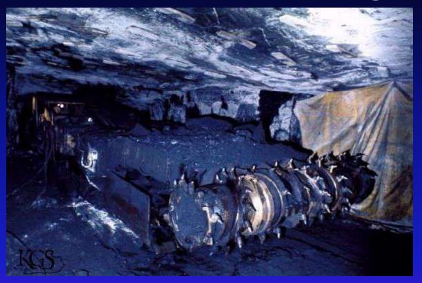
The machine that scrapes the coal seams with its rotating wheel of blades.
