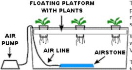
The water culture system is the simplest of all active hydroponic systems. The platform that holds the plants is usually made of Styrofoam and floats directly on the nutrient solution. An air pump supplies air to the air stone that bubbles the nutrient solution and supplies oxygen to the roots of the plants.
