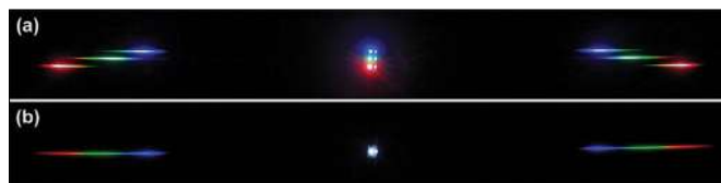
Fig. 8. Spectra of different LEDs as seen through the grating with 500 lines/mm: a) red, green, and blue LED spectra; b) white LED spectrum.
