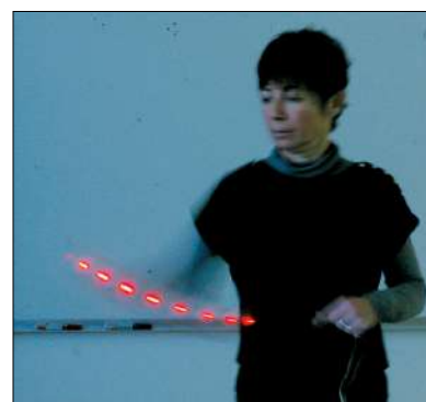
Fig. 4. Photo of light traces produced by a moving LED that is connected to an ac transformer.
