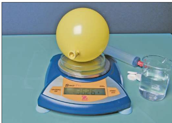
Fig. 4. Balloon on the scale. The tablets are inside and the balloon is expanding.
