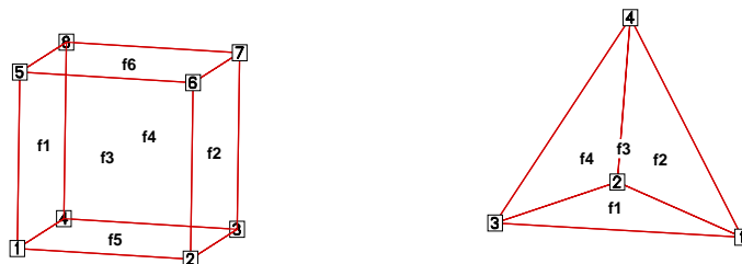
Figure 2-1. Examples of brick (left) and tetrahedron (right) face neighbors.
