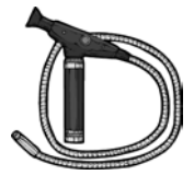
Fiber optic scopes can see around corners.
