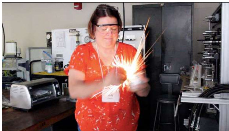
Fig. 2.25 White sparks and a loud crack should be produced when the spheres strike and slide past each other
