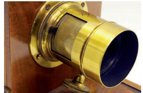
▲ This Voigtlander lens from the 1850s is equipped with slot for Waterhouse stops. A stop’s rectangular tab can be seen protruding from the side of this lens.
