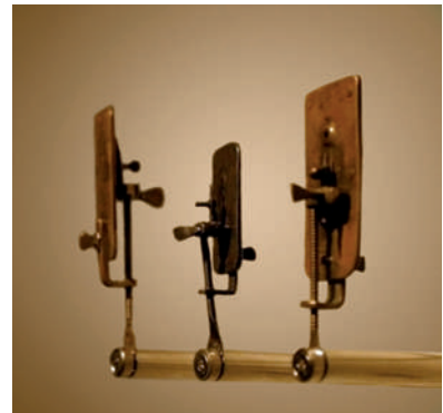
▲ These strange looking devices are Leeuwenhoek's original handmade microscopes. Of the hundreds he built during his lifetime, only a handful survive today. The lenses are tiny glass spheres located at the center of each handheld tool. The Museum Boerhaave for the History of Science and Medicine, Leiden, Netherlands.
