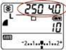
Many cameras display the current aperture and shutter speed settings on the monitor, in the viewfinder, or on a separate LCD panel when you press the shutter button halfway down.
