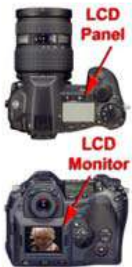
Many cameras have an LCD panel that displays settings and an LCD monitor that displays images and menus.
