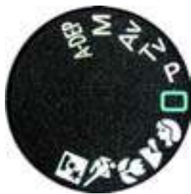
Many digital cameras have a mode dial you turn to select various exposure modes including automatic.
