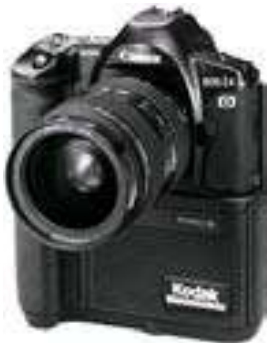
The Canon EOS DCS 3 digital camera was introduced in July 1995 and captured images containing 1.3 million pixels. It cost about $17,000.
