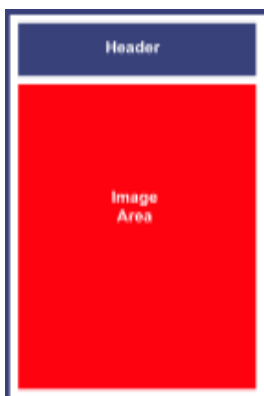
The header is an area of the file separated from the image data.
