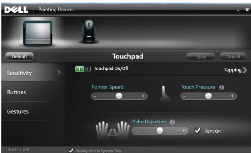
4. Adjust Pointer Speed, Touch Pressure, Palm Rejection or Set the Touchpad On/Off as desired.
