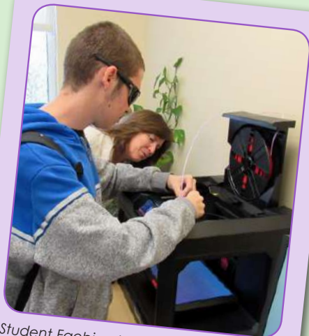
Student Faebian loads the raw materials (plastic filament strips) into a 3D printing machine as Librarian Ms. Amy Brody verbally guides him along the steps.
