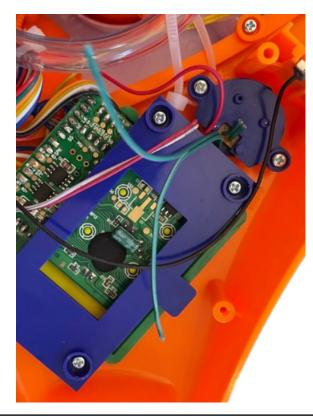
**4.** Take one side of the stereo extension cable and one side of the toy wire and twist to wrap the copper around each other.
