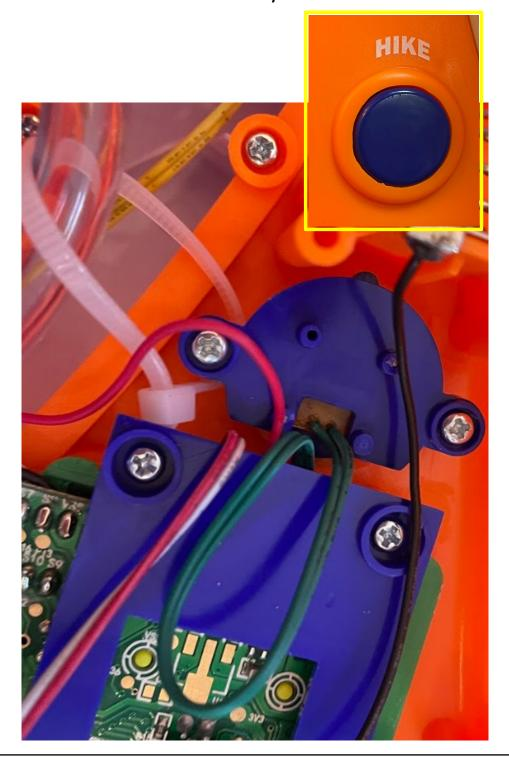
3. Use your scissors or wire cutter to snip the two green wires as close as you can to the back of the hike button, so the wires still lead to the circuit board.
