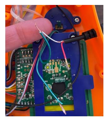
2. Strip the top of each wire to expose copper.
