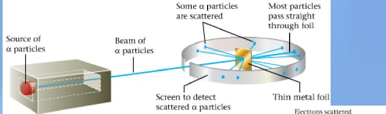
If the plum pudding model were correct, the α particles would have passed right through the foil.
