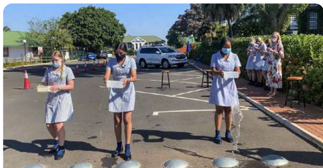
Figure 2 This shows the short course over which the girls moved to the stopping point. The speed of movement and deceleration are different for all three girls, which affected the amount of water that spilt out of the containers.
