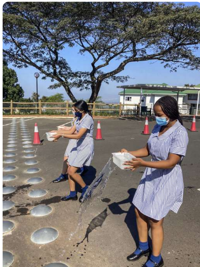
Figure 3 The girls each came to rest at slightly different times. The girl in the foreground of the picture has stopped completely and suddenly, so the water container also stops moving. The water in the container resists the change and carries on moving owing to its inertia, and therefore spills forwards out of the container. The girl in the centre has reduced speed more gently and spilled only a little water. The girl in the background decelerated even more gently and managed not to spill any water.
