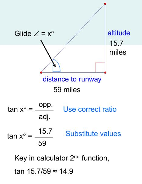
When the space shuttle's altitude is about 15.7 miles, the glide angle is about 14.9°.
