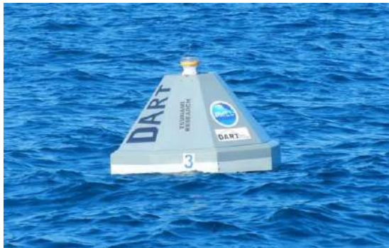
Figure 10-6 Deep-Ocean Assessment and Reporting of Tsunamis System (DART)
