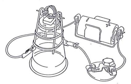
8. Place a magnet on the top of the inverted cup. underneath the coil. Turn the switch on and blow gently on the coil to help it get started.
