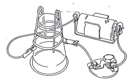
5. Next, begin to make the moving coil from the #28 wire. The wire has a thin coating of insulation on it called enamel, so you will need to sand off the insulation at the ends. This is so that the electricity can flow from the bare copper wire through the thin wire to the other bare copper wire.
