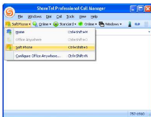
Figure 7-1 Activating SoftPhone from the Extension bar
