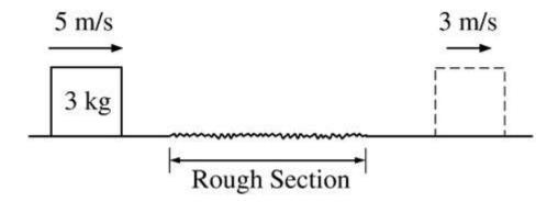
A block of mass 3 kg slides along a horizontal surface that has negligible friction except for one section, as shown above. The block arrives at the rough section with a speed of 5 m/s and leaves it 0.5 s later with a speed of 3 m/s.
