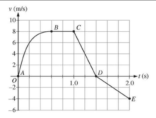
A cart is constrained to move along a straight line. A varying net force along the direction of motion is exerted on the cart. The cart's velocity v as a function of time t is shown in the graph above. The five labeled points divide the graph into four sections.
