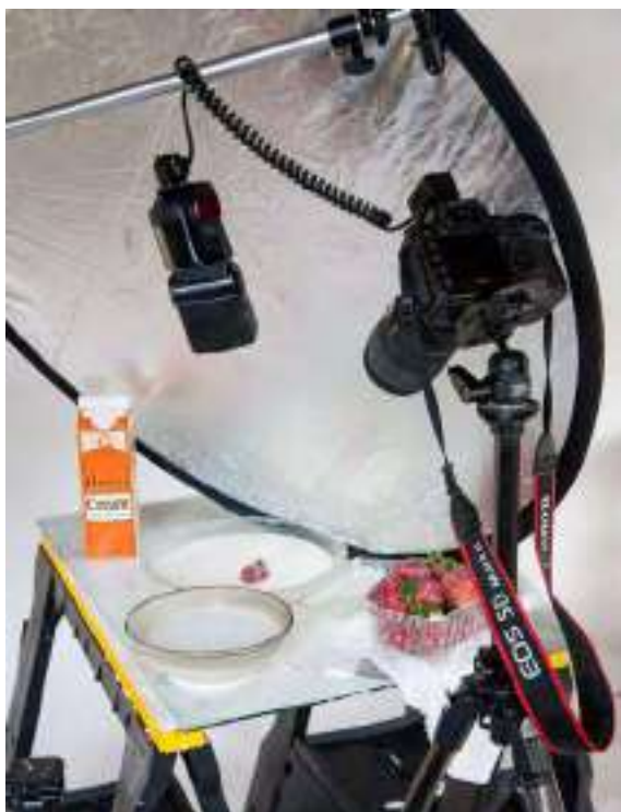
Figure 3-19: I used an off-camera flash sync cord to enable high-speed flash sync.
