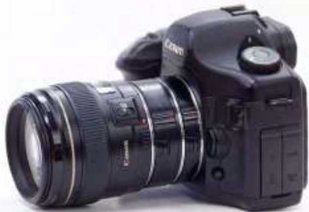
Figure 12-2: Extension tubes (such as the two in this picture) connect between the lens and camera, allowing you to focus closer.
