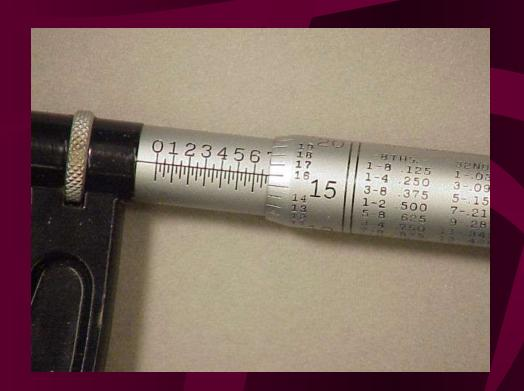
• Count the small lines between the long 6 line, and the edge of the thimble.
