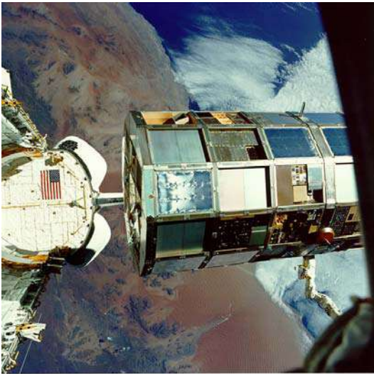
Figure 4: The LDEF, in orbit for 5.75 years, saw about 1 impact/m 2 which could have penetrated a typical 1.5 mm thick electronics box [4].
