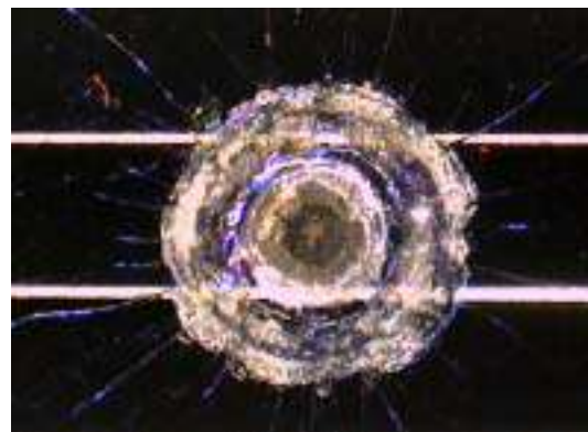
Figure 2. Meteoroid impact crater on a Solar Max solar panel; crater size: 3.5 mm, hole size .5 mm.
