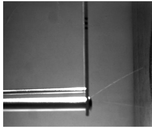
Figure 17: Image shows aluminum projectile captured as it struck the plate at 260 m/s.
