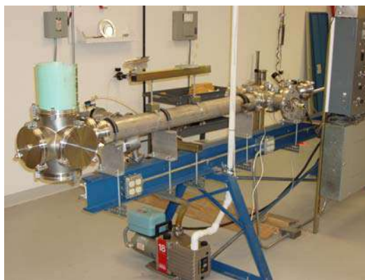
Figure 13: The CASPER LGG uses helium at 500-1000 psi to fire projectiles up to 800 m/s. A laser fan is used to determine the velocity of the projectile. The LGG was run under normal atmospheric pressure rather than under vacuum as in previous experiments.
