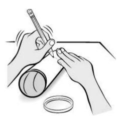
**5** The shorter bottom piece has a metal end. With the thumbtack, make a hole in the center of the metal.
