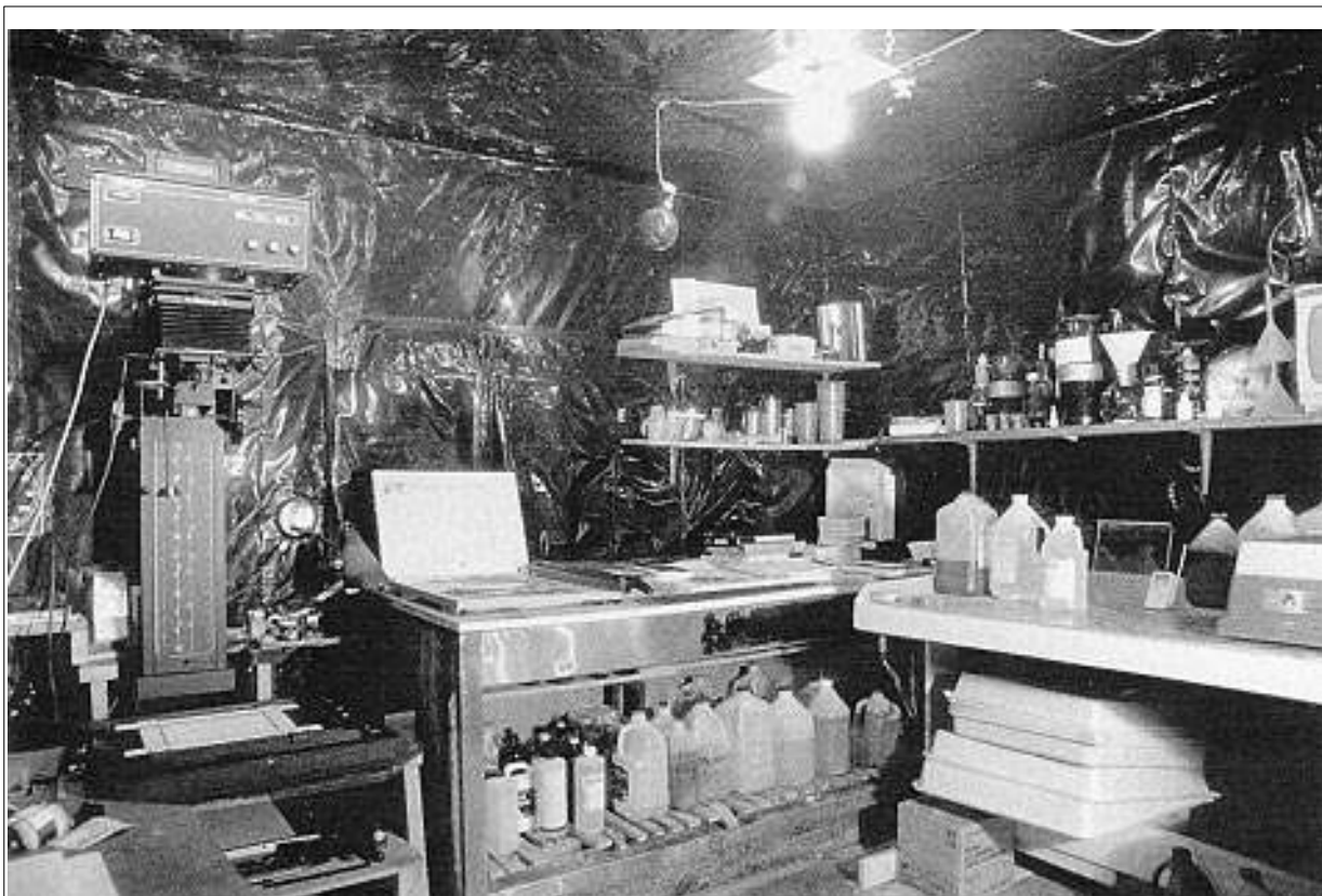
Figure 13-2 I mounted my enlarger as far from any wet materials as possible. I've never had chemical or water spots appear on prints during processing, and I hope I never do.
