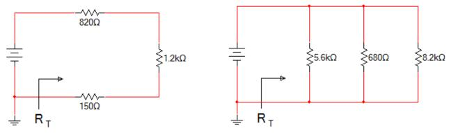
3. Using the laws of circuit theory, solve for  $R_T$ ,  $I_T$ ,  $V_{R1}$ ,  $V_{R2}$ , and  $V_{R3}$ . Be sure to put your answer in proper engineering notation and use the correct units.
