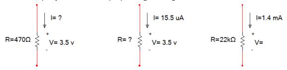
2. For each of the circuits shown below, calculate the value for  $R_T$ . Be sure to put your answer in proper engineering notation and use the correct units.
