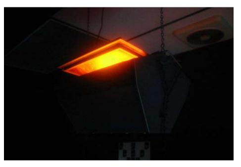
Red light provides safe light conditions to load photographic paper into a camera.
