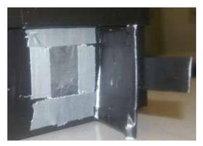
The shutter is the mechanical component of the camera system by means of which control the time interval of exposure is controlled. In this case, it's a manual shutter, moved by the person operating the camera.
