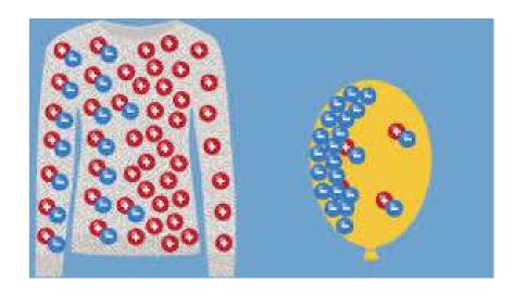
Two neutral objects, when rubbed together, can become charged by one object transferring its electrons to the other object
