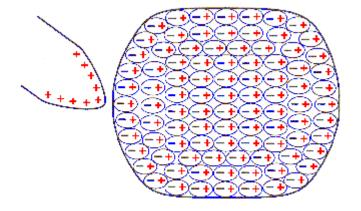
Even though no charge moves, the charges align themselves so that the negative charge of the insulator is near the positive charge of the charged rod
