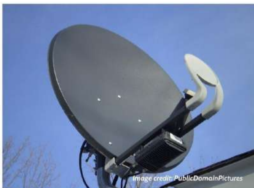
A satellite dish receives microwave radiation from a satellite thousands of miles above Earth, allowing TV companies to send programs to specific households.
