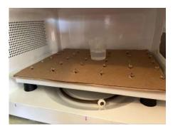
When you turn on the oven, some neon light bulbs will turn on and some will not. If you want to repeat this demonstration, do not run the oven for more than 10 seconds at a time. Replace the heated water with cold water, and then repeat the demonstration. If you don't see a clear pattern, reduce the amount of water in the container.
