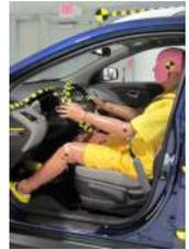
Engineers strategically place sensors on the crash test dummy in locations where people can be most impacted by a car crash. These include the head, neck, and chest. Data from these sensors help engineers identify and quantify how a person is impacted in these most likely injury locations or injury indicators of potential occupants.
