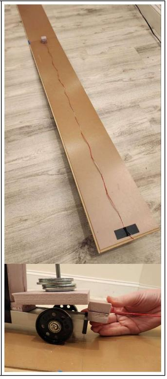
Note: A common mishap in data collection is for the brake string to get caught on something, like the corner of the ramp. To prevent that, we suggest bunching the string on the ramp behind the cart each time the cart is positioned, rather than letting it dangle over the end.
