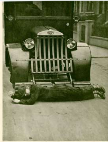
A "MAN-CATCHER." This safety device consists of three rollers attached to the bumper of the vehicle. Identify the rollers' track as individuals, they automatically drop to the ground and push it away.
