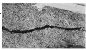
ground, as seen in the picture above. This crack was 150 feet long, 2-3 inches wide, and 2-3 inches deep when the photo was taken six weeks after the earthquake.
