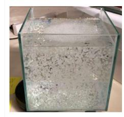
When liquid in a fish tank or a lava lamp is heated from below, the solid matter suspended in the liquid moves. We develop a model to explain the movement of material in the mantle. We analyze a video of a tank simulating the matter in the mantle to figure out what happens to the matter when heat is added. We observe convection in the tank and revise our model to represent it. We compare this model to tomography data and revisit our DQB. We figure out:
