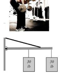
angle with the beam. Apply the conditions of equilibrium to the beam and use them to estimate the force that one primary back muscle (it is a complex system) exerts on the backbone and the force that the hinge (joint) exerts on the backbone on the left side. If you are having trouble, consult Example 8.7 on page 236 in the textbook. (Each year more than half a million Americans get serious back problems by lifting this way.)
