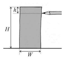
distance h where this transition happens, as precisely as possible. The coefficient of static friction between the block and the supporting surface is determined by the following mathematical representation:
