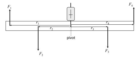
Four forces are exerted at different points on a meter stick (as shown in the diagram above) that is held up at its center of mass by a spring scale. The meter stick is in static equilibrium (not moving and not rotating). Write a mathematical expression (in terms of  $F_1$  to  $F_4$  and  $r_1$  to  $r_4$ ) for the rotational condition for static equilibrium about the pivot point shown in the figure. How
