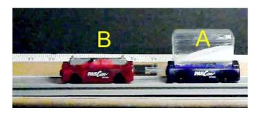
modeling clay, you adjust the total mases of the carts so they are both equal to 565 g. You push cart A so that it starts moving towards cart B (which is initially at rest). The carts collide. You take a video of the experiment and analyze it (watch the video
