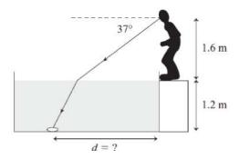
A ray from the eye to the coin is shown in the figure above.
