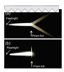
When you turn the foil around and repeat the experiment, the light beam reflects from the foil and no light passes through (see figure (b)).
