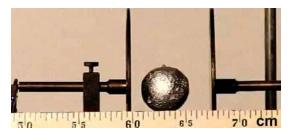
hanging on a nonconducting (insulating) string. The video is recorded at 600 frames per second. *Note*: if some charges are removed from the plate, the high-voltage source replaces these charges with new ones, so the potential difference between the plates remains constant.
