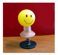
We modified the Jumper shown in the photo by gluing a square piece of cardboard onto its head. This also allowed us to launch the Jumper in the head-down position. The total mass of the Jumper is 6.0 g. Note that in each experiment, the spring was compressed an equal distance, 1.5 cm.
