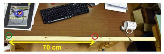
**Experiment** We held a mug somewhere close to the right end of the wooden plank (without touching the plank) and hit the mug with a spoon. The recorded signals are shown in the figure below. On the vertical axis you see the pressure and on the horizontal axis you see the time in milliseconds (m stands for milli).
