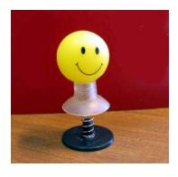
We modified the Jumper shown in the photo by gluing a square piece of cardboard onto its head. This also allowed us to launch the Jumper in the head-down position. The total mass of the Jumper is 6.0 g. Note that in each experiment, the spring was compressed an equal distance, 1.5 cm.
