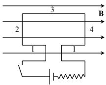
current flows around the loop in a clockwise direction. The loop resides in a uniform external magnetic field. Figure out the direction of the force exerted by the magnetic field on each side of the rectangular loop shown in the figures below.
