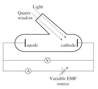
**b.** Use the simulation to observe that a UV light shines on the sodium cathode, the ammeter registers a current in the circuit independently of the intensity. How can you explain how UV light can cause the current? *Note*: A voltmeter has very high electrical resistance.
