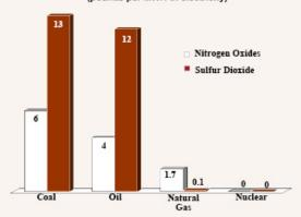
Power plant emissions only, not including small emissions from mining, transportation and refining or enriching fuel.
