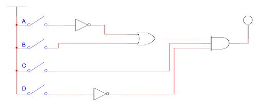
1) Convert the above A-I-O circuit to a **NOR only** circuit, then simplify by crossing out all redundant gates.
