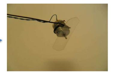
Twist the stripped ends of electrical wire onto the motor terminals. Wrap the wires around the coat hanger until they reach the battery, slip them under the rubber band and connect them to the battery. The motor should start spinning!
