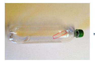
Trace and cut an oval out of a plastic bottle or cup. This will be your propeller. Poke a hole in the middle to attach to the motor shaft.
