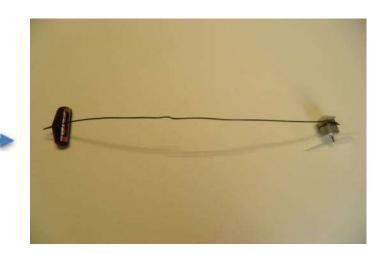
Attach a battery to the other end of the coat hanger wire with a thick rubber band.
