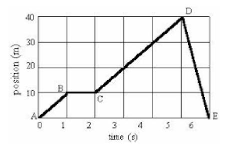
Determine the velocity (slope = rise/run) for each segment of the graph. (A-B, B-C, C-D, D-E).
